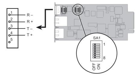
Set the SA1 switches to select the four wires configuration with termination:
